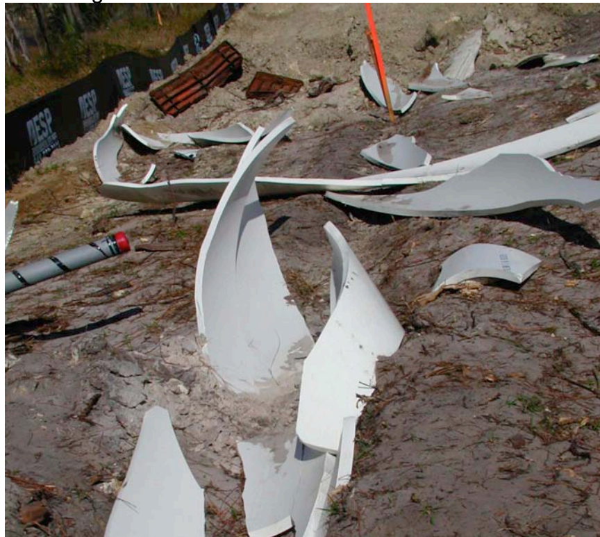
Figure 1 – RCP Field Failure in 30" DR 25 PVC
