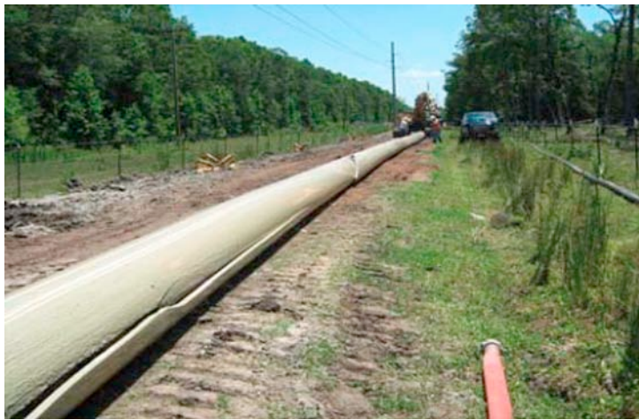
Figure 2 - RCP Field Failure - 20" DR 18 PVC Pipe
