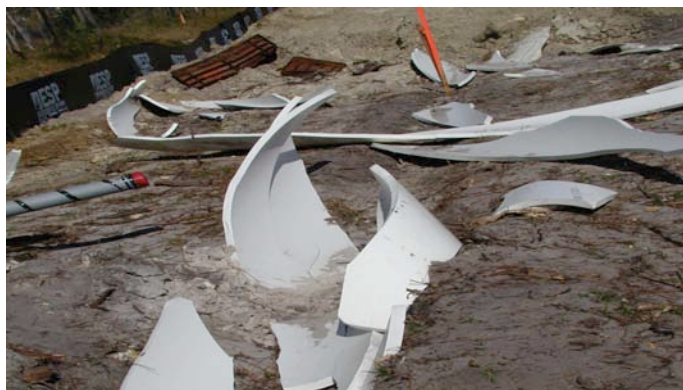
Figure 1 – RCP Field Failure - 30" DR 25 PVC Pipe
