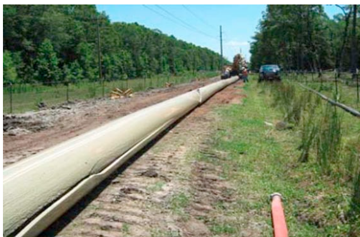
Figure 2 - RCP Field Failure - 20" DR 18 PVC Pipe
