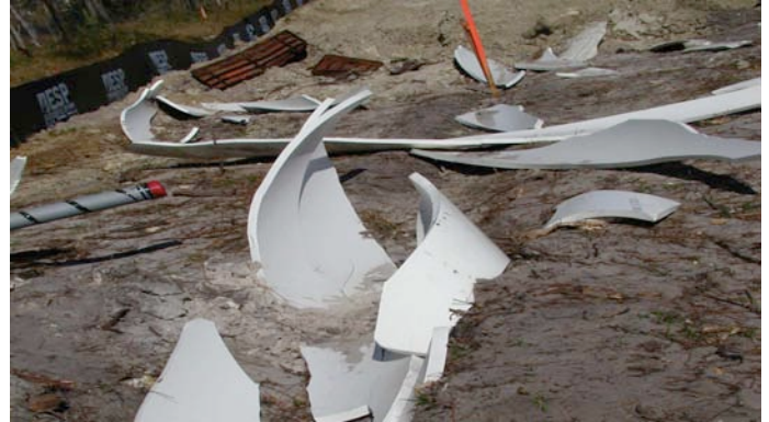
Figure 1 – RCP Field Failure - 30" DR 25 PVC Pipe
