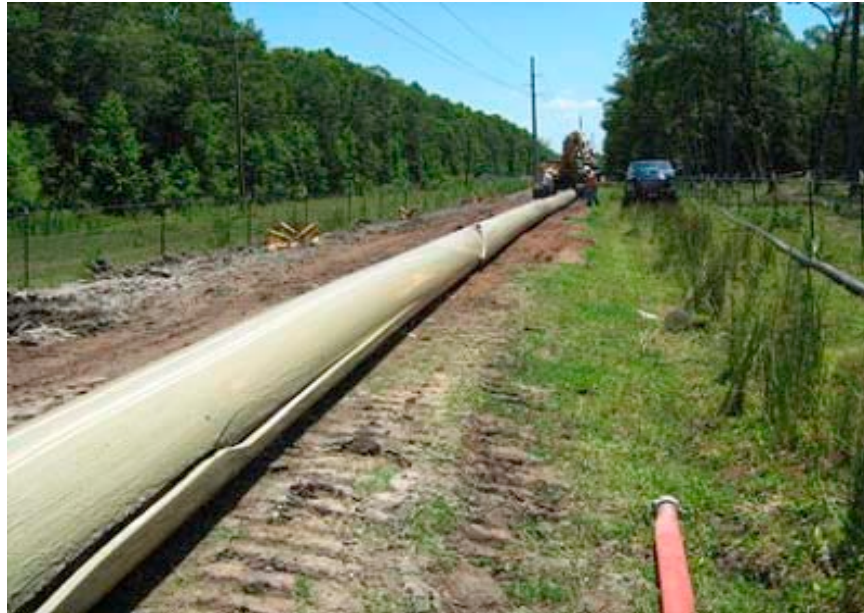
Figure 2 - RCP Field Failure in 20" DR 18 PVC Pipe
